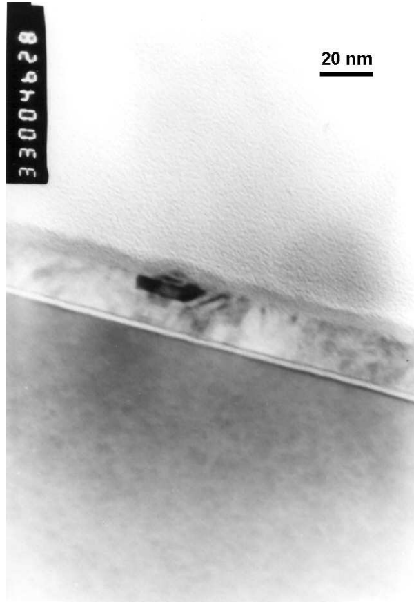
Figure 51: TEM cross section of a 1.9nm oxide resulting of 10 minutes of dry oxidation at 725°C.
